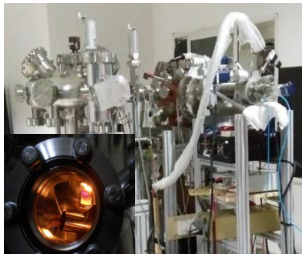
Figure: Setting up of a thin film cluster vacuum system with the capability evaporate ultra clean thin films of metal and oxides (As shown in the inset)
