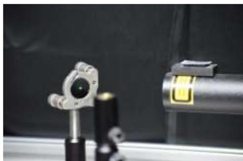
The cuvette-FCS setup uses a green Helium-Neon laser (picture left). The laser is zoomed using a telescope and aligned precisely using several mirrors before being focused by the ELWD objective. When the laser beam excites the molecules, they emit fluorescence. This is detected by avalanche photodiodes (APD). APDs are very sensitive; it can detect even a single photon. Dr. Bankanidhi Sahoo, a postdoctoral fellow and Timir Baran Sil, a graduate student figured out that the quality and the precise
