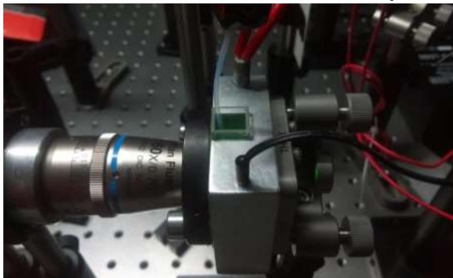
*FCS set up with the cuvette*
