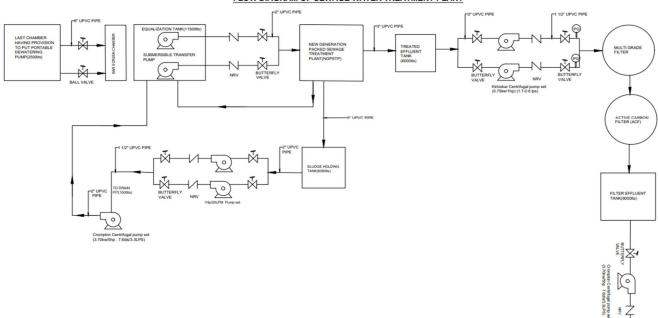
FLOW DIAGRAM OF SEWAGE WATER TREATMENT PLANT
