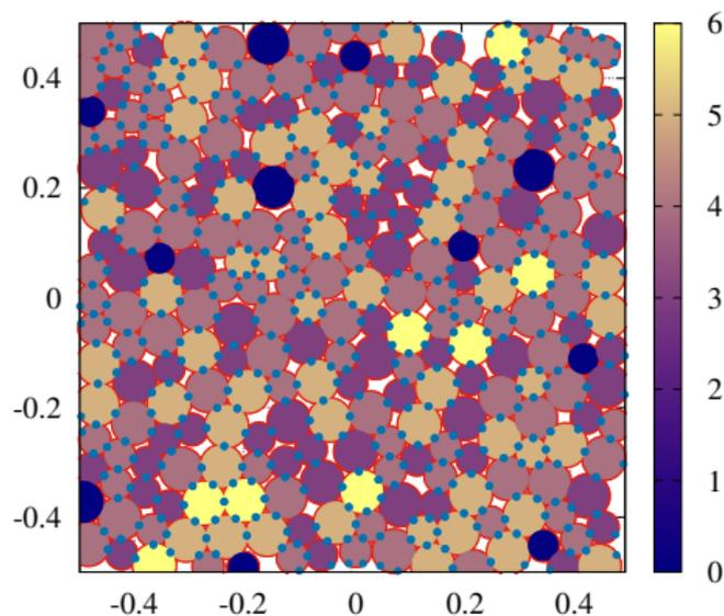
**Figure:** A jammed packing of 256 bidispersed frictionless disks coloured according to their contact numbers.
