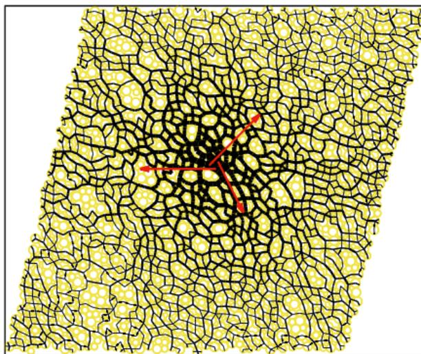
The response of a sheared system of soft frictional disks to applied body forces (represented by red arrows) with Lees-Edwards boundary conditions at global shear  $\gamma = 0.43$ . The response provides characteristic signatures of the emergence of "force chains" along the compressive direction.
