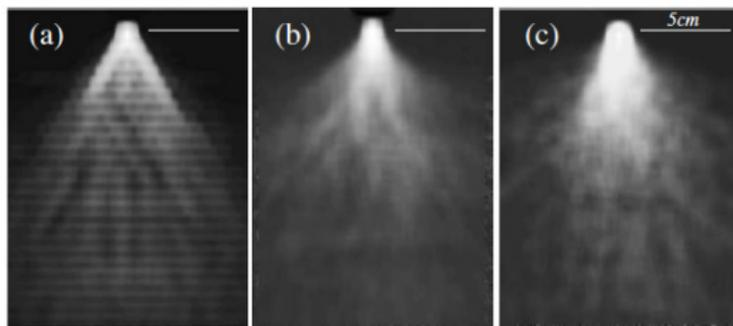
**Mean response** of a 50 g point force for (a) a uniform hexagonal packing of disks, (b) a bimodal packing of disks (c) pentagons. Ref: J. Geng, D. Howell, E. Longhi, R. P. Behringer, G. Reydellet, L. Vanel, E. Clément, and S. Luding, *Phys. Rev. Lett.* **87**, 035506 (2001).
