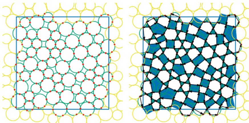
**(Left)** A jammed packing of bidispersed frictionless disks with periodic boundary conditions. **(Right)** The same configuration with the associated grain polygons (white) and void polygons (blue).
