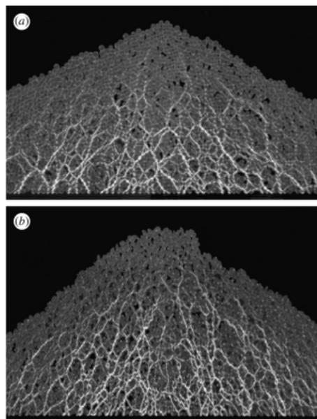
Inhomogeneous stress transmission in granular piles made with (a) disks and (b) elliptic cylinders. Ref: I. Zuriguel, T. Mullin, *Proc. Royal Society A* 464, 2089 (2008).
