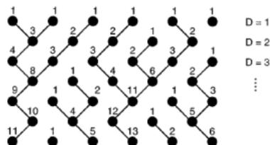
Schematic diagram showing the paths of weight support for a two-dimensional system in the  $q_{0,1}$  limit where each site transmits its weight to exactly one neighbor below. The numbers at each site are the values of  $w(i, D)$ .
