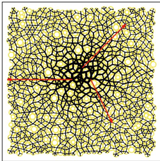
The response of a system of soft disks to applied body forces (represented by red arrows). The inhomogeneous nature of the stress response is clearly illustrated.
