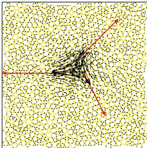
The response of a system of soft grains to applied body forces. The black arrows represent the changes in the contact force vectors in response to the imposed body forces (red arrows).
