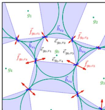
The height fields  $\{\vec{h}\}$  are associated with the void polygons (shaded light blue). The forces are represented by (bidirectional) arrows.
