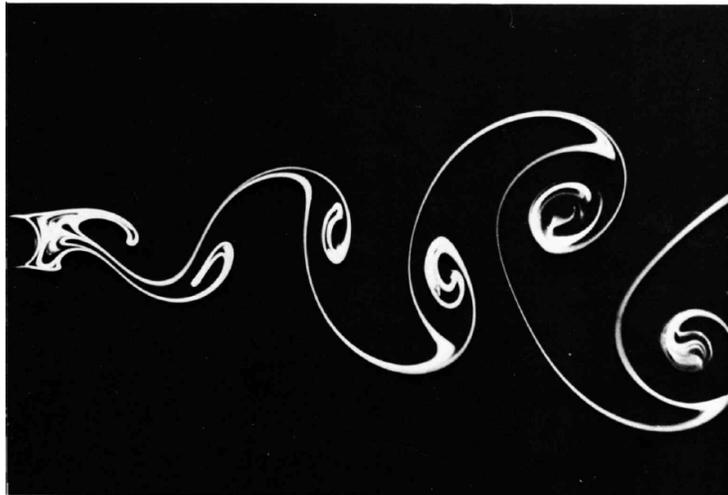
Figure 1.6: Flow past a cylinder at  $Re = 0.16$ . The photograph is taken from the book by Frisch [8] and is the same as Fig. 94 on page-56 of the book by Van Dyke [18].
